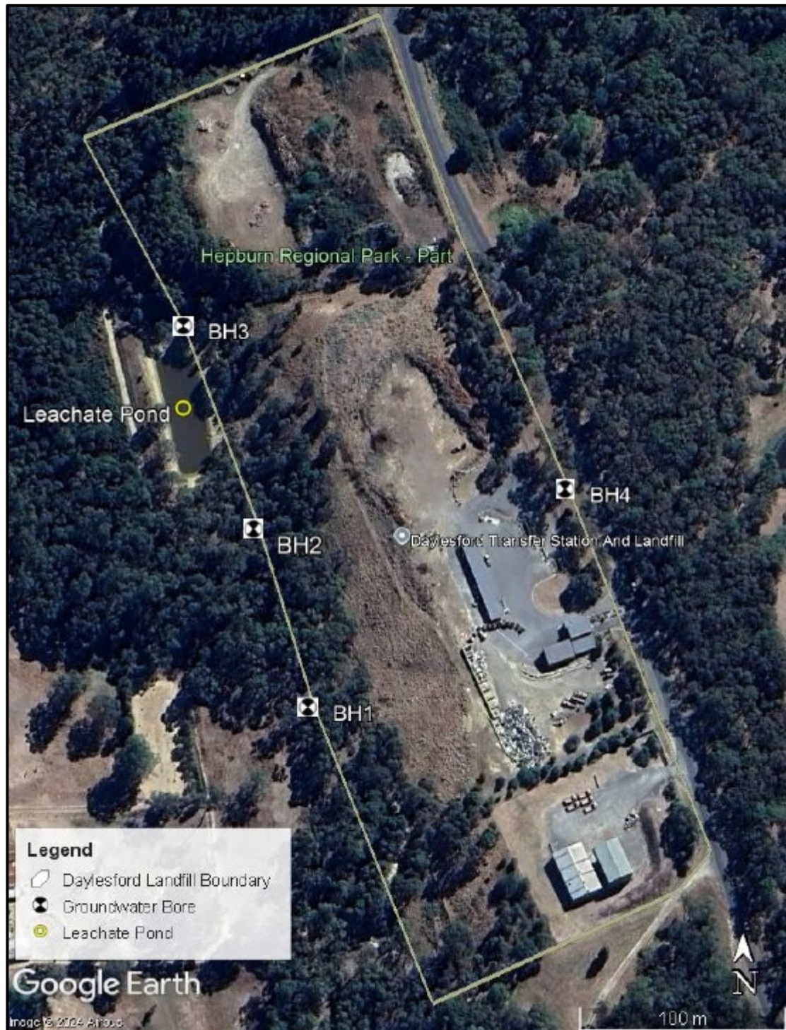
Figure 2: Groundwater Monitoring Well Locations
